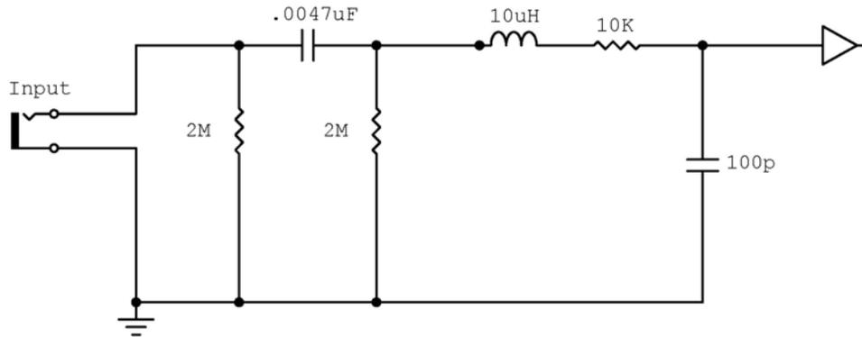
Figure 3: Equivalent Input Stage
